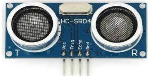
Gambar 1. Sensor Ultrasonik HC-SR04.
